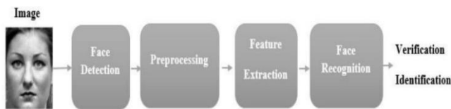
Fig. 3 Structure of Face Recognition System[3]
